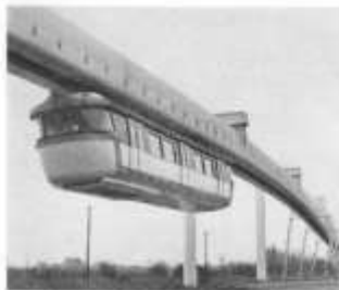
34. The experimental monorail track of S.A.P.A.S.A. TRANSPORT near Paris. The car is suspended from rubber tyre bogies running inside the track, and operation is thus silent and impervious to weather.
